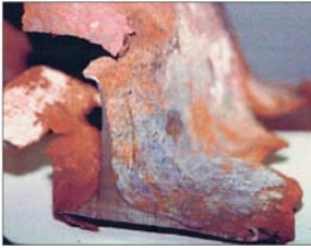
WTC steel sample after hot corrosion attack. FEMA, Appendix C
